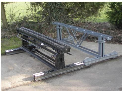
The secondary transporter has been finished too (**See Picture Left**), with a new adjustable frame fabricated, new wheels and locking mechanism installed, complete with a couple of coats of sprayed, grey paint. The steaming bays have also been straightened, painted and the turntable modified so the locking mechanism, actually locks in place! In fact all in all it is looking very tidy out the front now.
